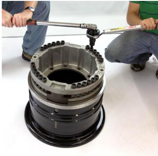
Tightening Hub Adapter to Transducer Bolts with Torque Wrench and Torque multiplier (note: picture does not show mounted tire. Normal Install will have tire already mounted to Rim)
