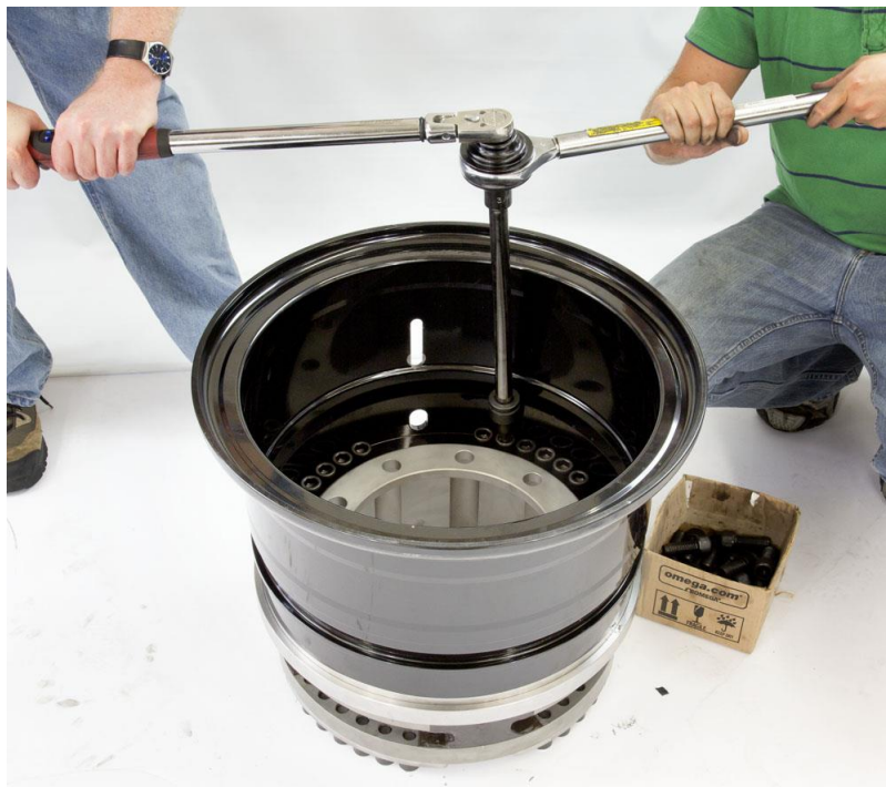
Tightening Inner Transducer Bolts with Torque Wrench and Torque multiplier (note: picture does not show mounted tire. Normal Install will have tire already mounted to Rim)
