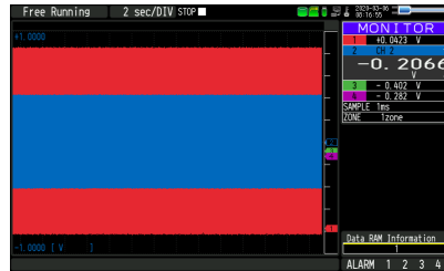
CH2 is active CH. The waveform of CH2 is displayed on the top, so you can visually recognized it.
