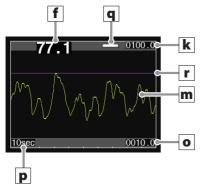
The screen will appear as follows when the peak to peak hold or peak and bottom hold function is active.
