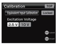
Select the bridge voltage to supply to the strain gauge transducer.
