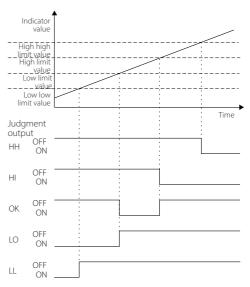
When set to OK/LL/LO/HI/HH, all are assigned to high limit (when Standard Comp. Output Pattern setting)
