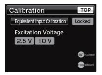
Use the  $\blacktriangleleft$  and  $\blacktriangleright$  buttons to select TOP, and press the ENT button to return to the Home Screen.
