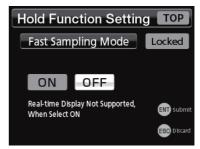
While a hold is being executed, the following screen appears and the hold value cannot be checked in real time.
