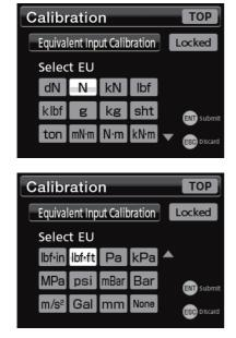
Options: dN,N, kN, lbf, klbf, g, kg, sht, ton, mN·m, N·m, kN·m, lbf-in, lbf-ft,Pa,kPa, MPa, psi, mBar, Bar, m/s<sup>2</sup>, Gal, mm, none
