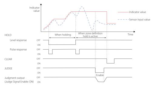
When holding, the peak value is reset by pressing the CLEAR (ESC) button or by a control input terminal CLEAR signal becoming ON.
