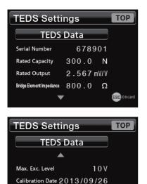
Press the ESC button to exit TEDS data display mode.
