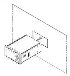
4 Attach the left and right panel attachment fixtures that were removed in step 2 to the unit from behind and fix them in place.
