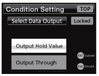
Select Data Output has the following two options. The hold value is output in coordination with the display. The input is output as is.
