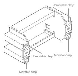
2 Push the adapter on to the DIN rail at an angle and connect it.
