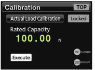
Check the load calibration results. If there are no problems, press the ENT button to confirm them.
