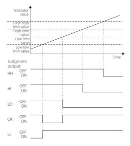
When set to LL/LO/HI/OK/HH, one is assigned to high limit and three are assigned to low limit (when Standard Comp. Output Pattern setting)
