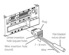
1 Remove 7–8 mm of the covering from the wire being connected, and twist it so that the tip does not come apart.
