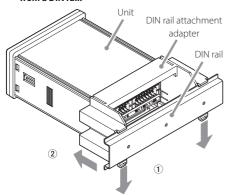
2 Open the four clasps on the left and right sides that hold the attachment adapter and the unit together, and remove the attachment adapter from the back of the unit.
