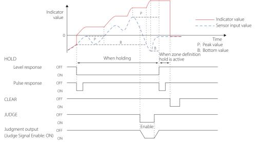
When holding, the peak to peak hold value is reset by pressing the CLEAR (ESC) button or by a control input terminal CLEAR signal becoming ON.
