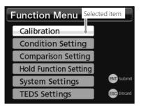
2 Use the ▲ and ▼ buttons to select the setting item, and press the ENT button to open the setting screen.
