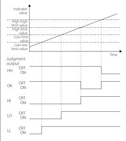
When set to LL/LO/HI/HH/OK, all are assigned to low limit (when Standard Comp. Output Pattern setting)
