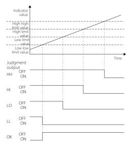
When set to LL/OK/LO/HI/HH, three are assigned to high limit and one is assigned to low limit (when Standard Comp. Output Pattern setting)
