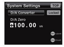
Use the  $\blacktriangleleft$  and  $\blacktriangleright$  buttons to change the selection, and use the  $\blacktriangle$  and  $\checkmark$  buttons to change the value.
