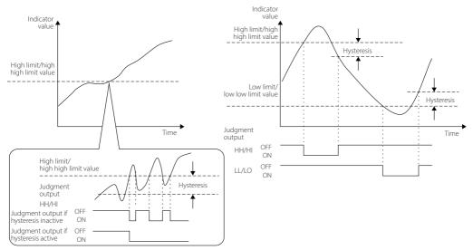
Judgment output conditions (when Comp. Output Pattern is set to Standard Output)
