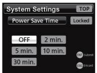
Use the  $\blacktriangleleft$  and  $\triangleright$  buttons to change the selected option, and press the ENT button. When there are multiple selections, pressing the t button when an option at the right end of a line is selected will select the option at the left end of the next line. A confirmed item will be shown with a green border.
