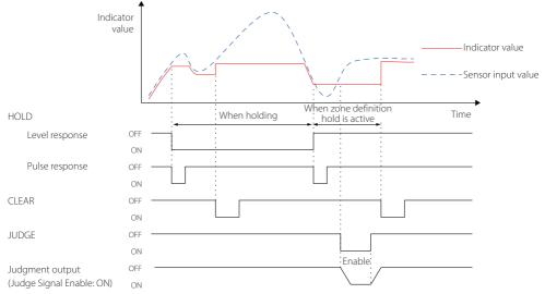
When holding, the bottom value is reset by pressing the CLEAR (ESC) button or by a control input terminal CLEAR signal becoming ON.
