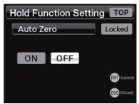
ON: automatically execute the Digital Zero function when a hold starts
