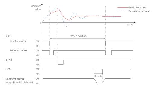
Even during the HOLD interval, if the maximum average calculation time is exceeded, average hold will end. If Zone Definition is set to ON, the average value is held at that point (page 69).
