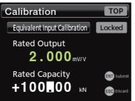
2 Move the cursor to the digit where you want to show the decimal point, and press the ▲ or ▼ button until the decimal point is shown.
